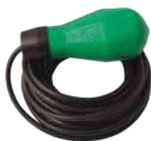
Floating switch for heavy waste water applic. Micro Switch 10(4)A Neoprene Cable H07RN-F 3X1 Counter-weight integrated
