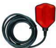
Floating switch for clean water Micro Switch 10(4)A PVC Cable H05VV-F 3X1MMQ
